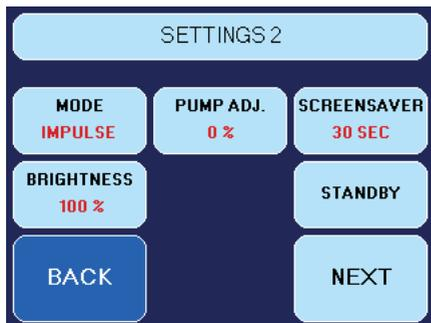
To open the Settings 2-screen, press **SETTINGS** at the main screen and, on the following Settings 1-screen, **NEXT**. The shown screen appears.
