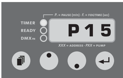
Adjusting of the output/pump in steps of 1% (1-99%)
